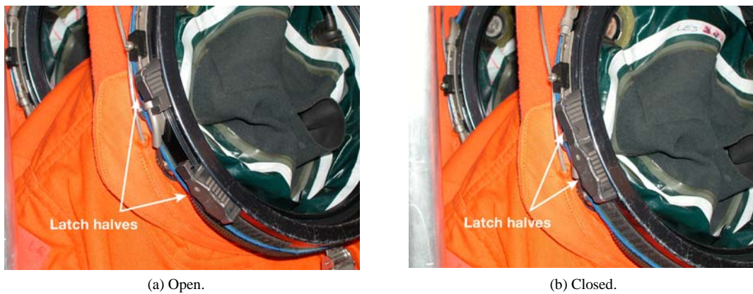
Figure 3.2-5. Example of neck ring latch.
