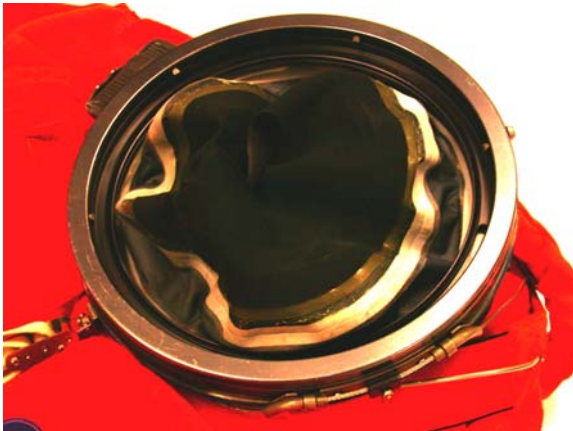
Figure 3.2-2. Example of neck ring.
