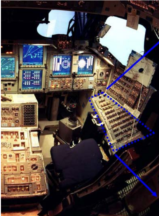
Figure 3.4-10. Location of the R2 panel. [Picture from the Shuttle Training Simulator]
