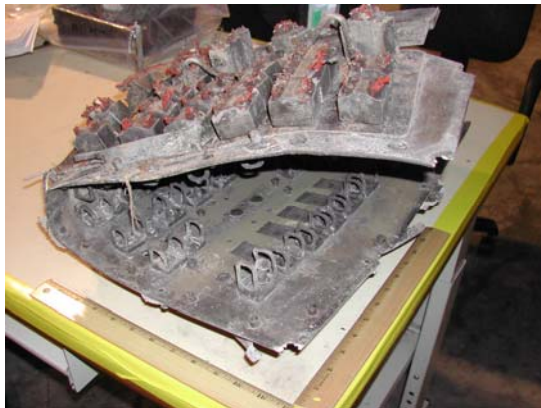
Figure 3.3-3. Recovered R2 panel from Columbia.
