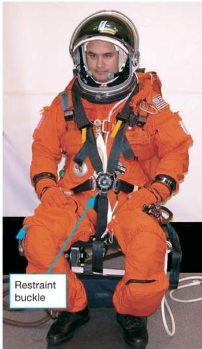
Figure 3.1-39. *Demonstration of the five-point seatbelt buckle.*
