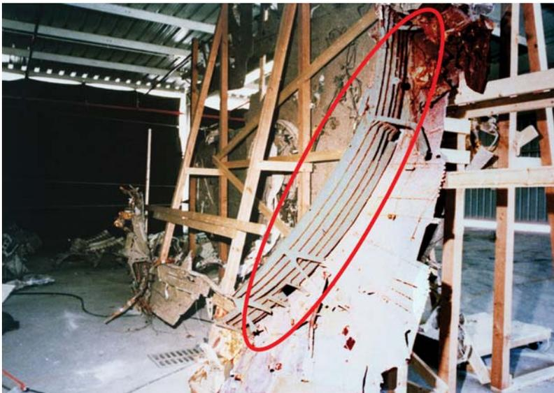
Figure 2.2-30. Recovered X<sub>o</sub> 576 bulkhead of the *Challenger* crew module showing a portion of the X<sub>o</sub> 582 ring frame bulkhead (circled in red).
