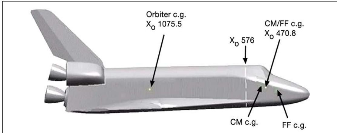
**Figure 1.1-28. X-axis center-of-gravity locations for the intact orbiter, the crew module, the forward fuselage, and the forebody (crew module plus forward fuselage). The  $X_o$  576 is the aft bulkhead of the crew module.**
