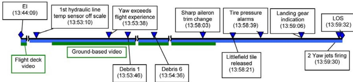
**Figure 1.1-8. Phase 2 timeline with key events.** Green bars represent times when video data are available. Blue bar represents when the Modular Auxiliary Data System/orbiter experiment (MADS/OEX) recorder data, and voice and telemetry transmissions are available (throughout this phase).
