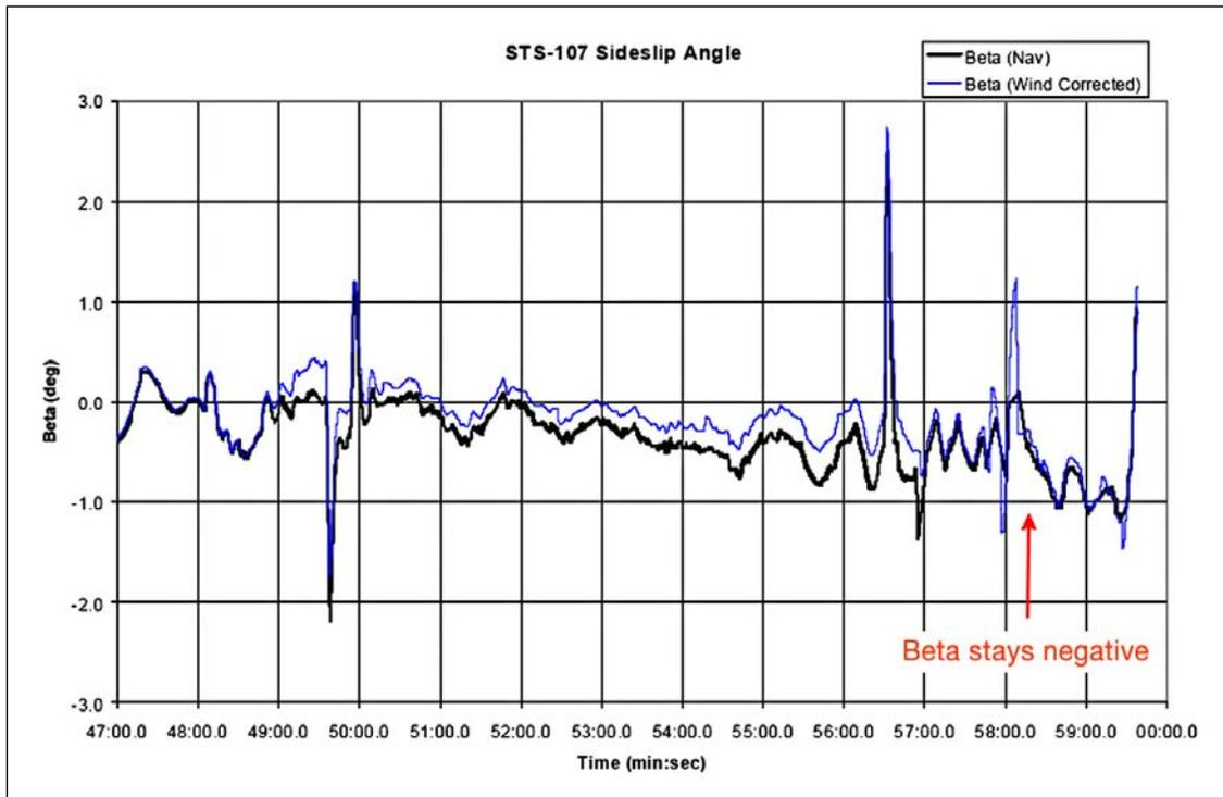
Figure 1.2-20. STS-107 sideslip angle vs. time.<sup>4</sup>
